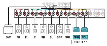
\* The surround Dolby or back Dolby speakers can be connected instead of the front Dolby speakers. In this case, set the Dolby Atmos Enabled speakers to be connected under "Height" - "Layout" in the menu. (12) p. 229)
