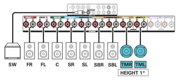
\* The top front or top rear speakers can be connected instead of the top middle speakers. In this case, set the ceiling speakers to be connected under "Height" - "Layout" in the menu. ( pp. 229)
