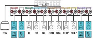
\* The height speakers, ceiling speakers and Dolby Atmos Enabled speakers can be connected to the HEIGHT1 speaker terminals. Set the speaker to be connected from "Height" - "Layout" in the menu. (1287 p. 229)
