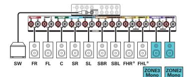
\* The height speakers, ceiling speakers and Dolby Atmos Enabled speakers can be connected to the HEIGHT1 speaker terminals. Set the speaker to be connected from "Height" - "Layout" in the menu. (127 p. 229)
