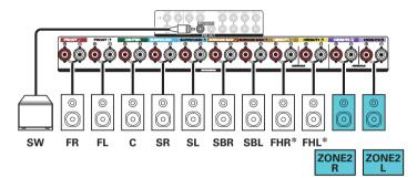
\* The height speakers, ceiling speakers and Dolby Atmos Enabled speakers can be connected to the HEIGHT1 speaker terminals. Set the speaker to be connected from "Height" - "Layout" in the menu. ( ) 229)
