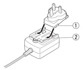
Align the ① guide with the ② guide and press it down in the arrow direction until it clicks.
