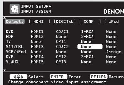
**4 Press ENTER, then use  $\triangleleft \triangleright$  to select the input terminal to be assigned.**
