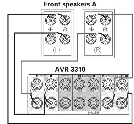
When in the "Front A Bi-Amp" and "Front B Bi-Amp" modes, the same signals are output from the front speaker terminals and the AMP ASSIGN terminals.
