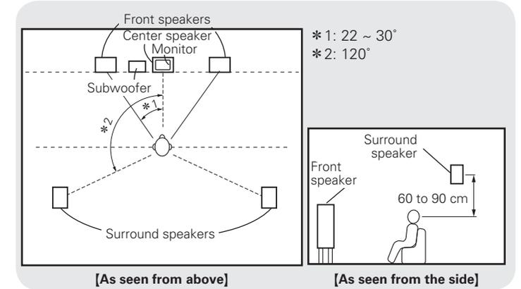
Installing/Setting the Speakers
