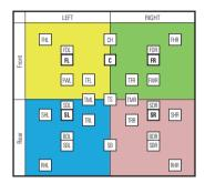
For example, if Subwoofer = 2 spkrs and Subwoofer Layout = Left/Right, Subwoofer Left (Subwoofer 1) plays the bass of the speakers in the Left area which includes FL/SL and Subwoofer Right (Subwoofer 2) plays the bass of the speakers in the Right area which includes FR/SR.
