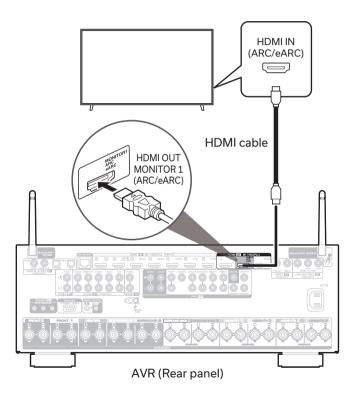
Using a high quality HDMI cable\*, connect one end to the HDMI port labeled "eARC" or "ARC" on your TV. Connect the other end to the HDMI OUT MONITOR 1 port on your AVR.
